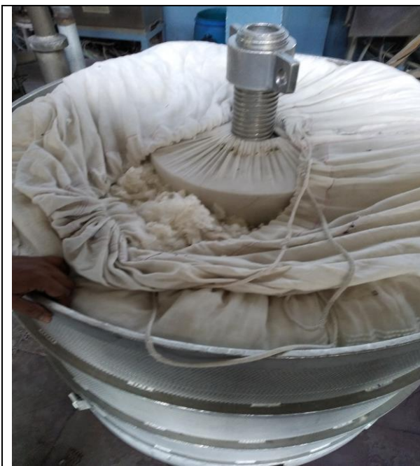
Photo: Perforated carrier with wool fibres loaded
